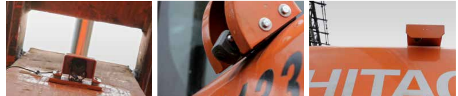
Left: Camera inside boom to monitor the working area Centre: Camera to monitor the vehicle's sides Right: Camera to monitor the vehicle's rear area
