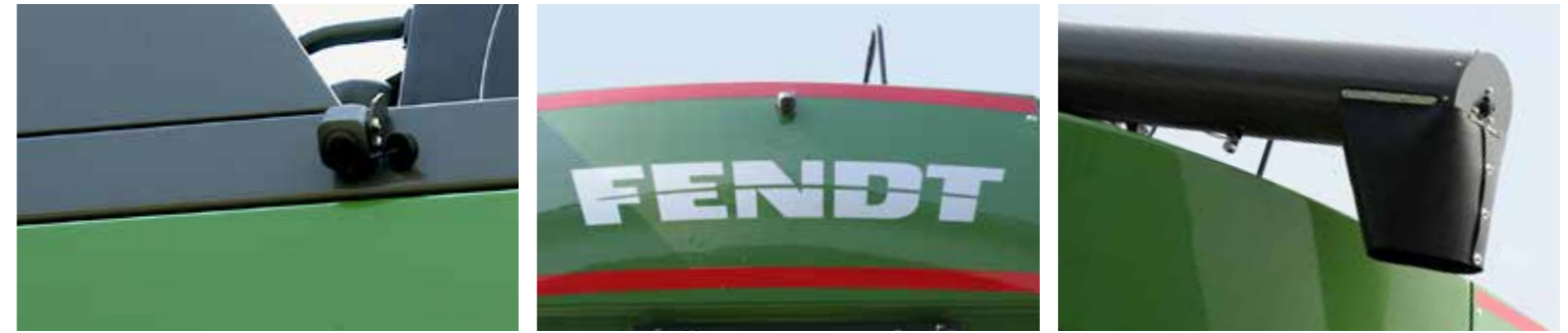
Left: Camera to monitor the vehicle's sides Centre: Camera to monitor the vehicle's rear area Right: Camera to monitor the vehicle's unloading spout
