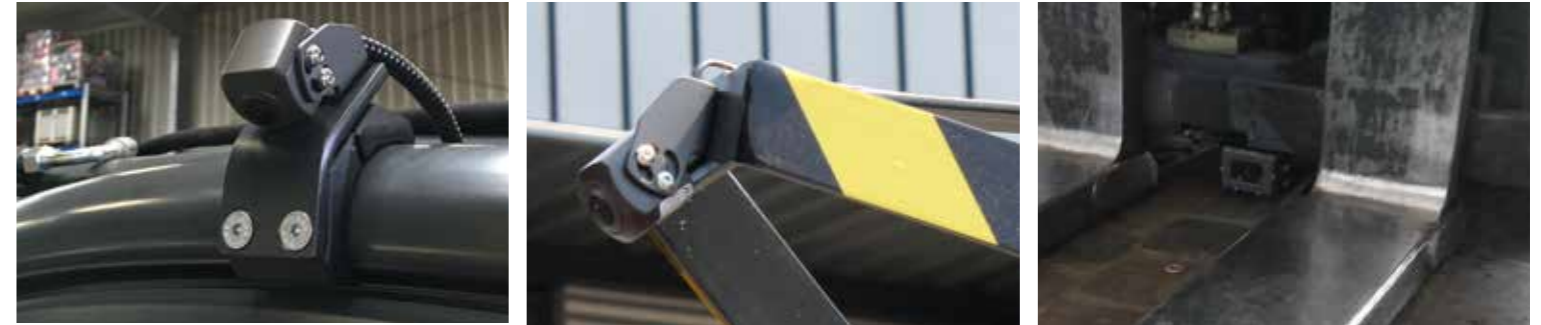
Left: Camera to monitor the vehicle's sides Centre: Camera to monitor the vehicle's rear Right: Camera to monitor the forklift truck
